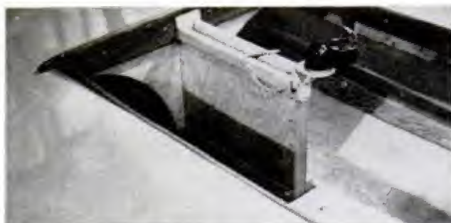
ALUMINUM ANGLE BRACKET holds cam cleat and the pin on a chain to hold daggerboard in down position
